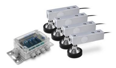
Ideal for creating platforms with 4 load cells of various sizes and capacities. The kit is made up of 4 350 Ohm IP67 nikel-plated load cells, OIML and NTEP approved, together with adjustable resting feet and an equalisation box.
